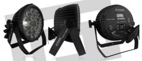
The new Encore Professional Lighting AuraPar<sup>™</sup> 18HEX IP is an IP65 rated Par featuring (18) 12 watt 6in1 (RGBAWU/V) Flicker Free LEDs rated at an average 100,000 hours. This fixture provides a 25° beam angle, electronic strobe/dimming (0-100%), 5 dimming curve modes, dual yoke hanging bracket / floor stand, IP rated power in & through, IP rated DMX in & through, 5 DMX channel modes, convection cooling for no-noise / fan-less operation, and heavy duty die-cast aluminum exterior build.
