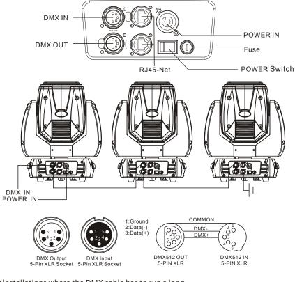
For installations where the DMX cable has to run a long distance or is in an electrically noisy environment, such as in a discotheque, it is recommended to use a DMX terminator. This helps in preventing corruption of the digital control signal by electrical noise. The DMX terminator is simply an XLR plug with a 120  $\Omega$  resistor connected between pins 2 and 3,which is then plugged into the output XLR socket of the last fixture in the chain. Please see illustrations below.
